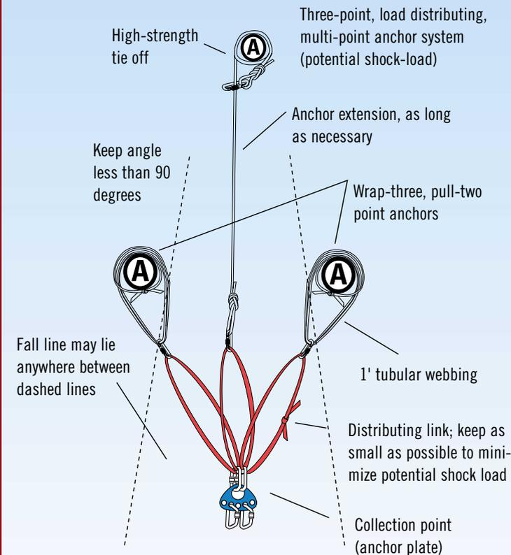
never exceed 90 degrees. Multi-point anchors are most often two-point anchors, but can incorporate three- or four-point anchors.
