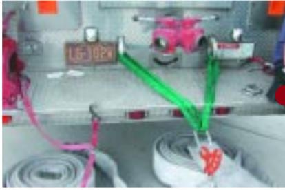
**You can use apparatus for anchor points, but be sure to use approved structural elements. Chock the wheels and post a guard to prevent anyone from operating the truck while it's being used as an anchor.**
