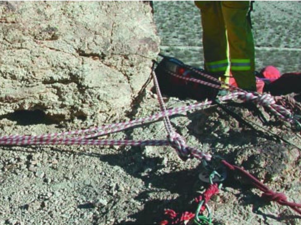
This anchor was set up with an entire 200', ½" rope. The rope was doubled and then doubled again. The four strands of rope were wrapped around a large rock outcropping. The end result had two loops for the working line and two loops for the belay line. It was bomber.
