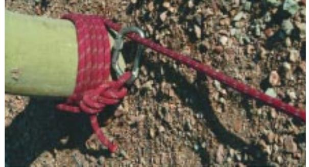
An excellent single-point anchor to set up a fixed-line for rappel or highline is the high-strength-tie-off (sometimes referred to as the tensionless hitch). Four to six wraps of rope provide enough friction to prevent the knot from having any tension on it, but it's not well suited to attach a system to.
